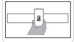
If you do not know the position of your NFC antenna, slightly move the smartphone in a circular motion over the Smart Touch logo until the App confirms the connection. In order for the data transfer to be successful, it is essential TO KEEP THE SMARTPHONE ON THE DASHBOARD DURING THESE THE FEW SECONDS OF PROCEDURE; a message on the device will inform about the correct outcome of the operation and advise you when it is possible to move the smartphone away.
